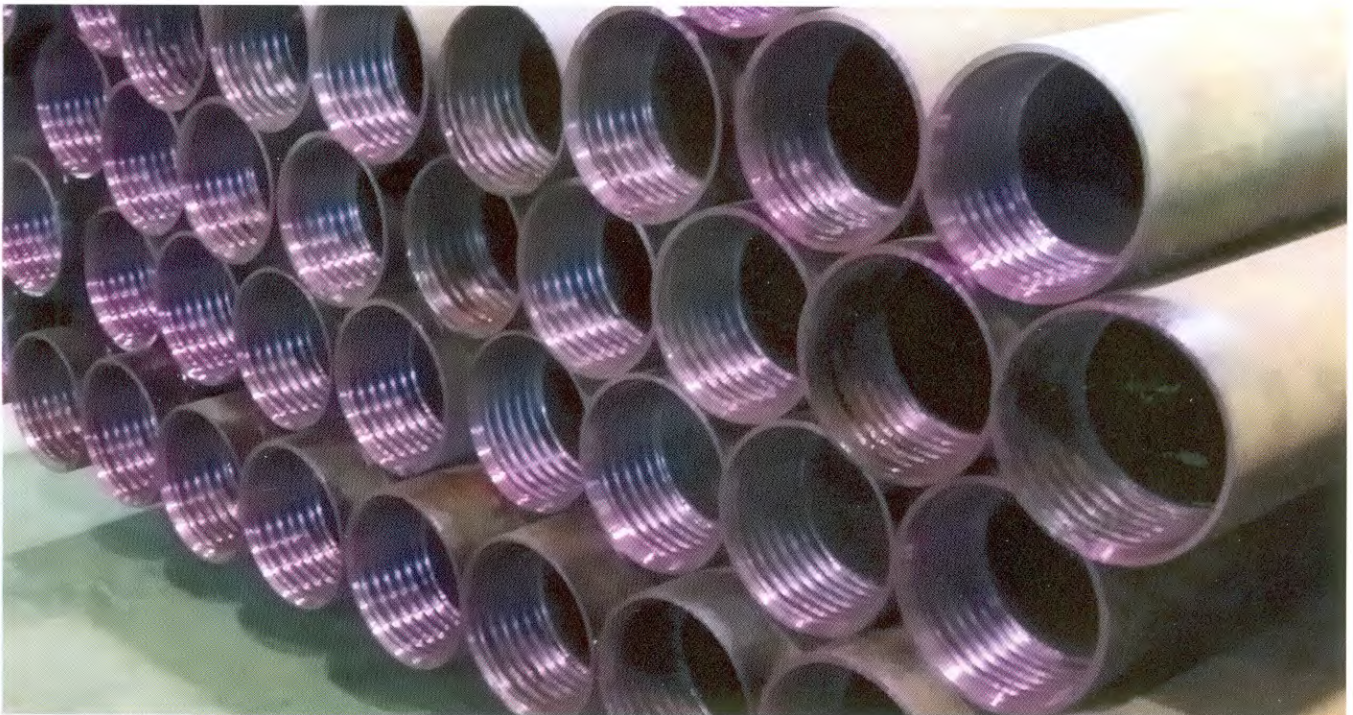
Example of anti-rust paint.
